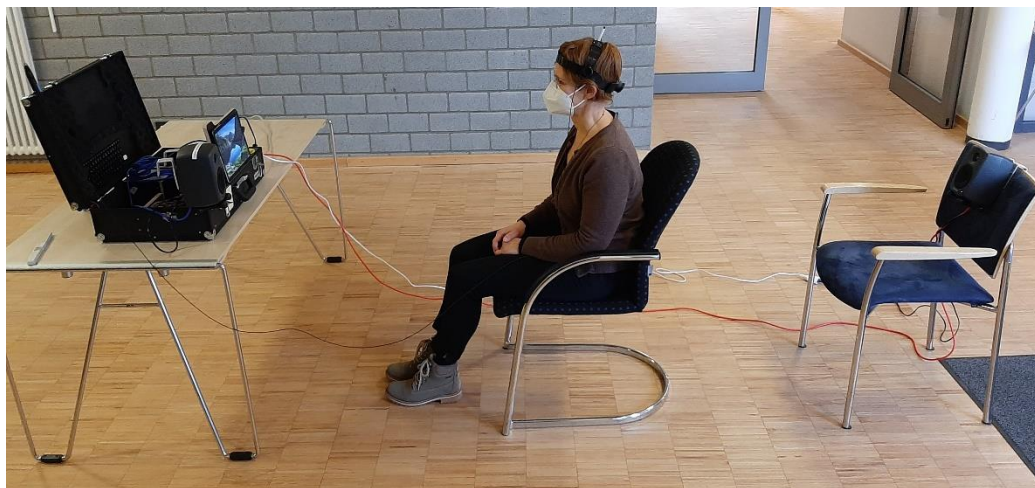
Figure 4. The setup used for the Oldenburg sentence test. Stimuli are presented from two loudspeakers placed in front of and behind the participant. A microphone mounted on the top of the participant's head monitors the sound pressure levels presented.
