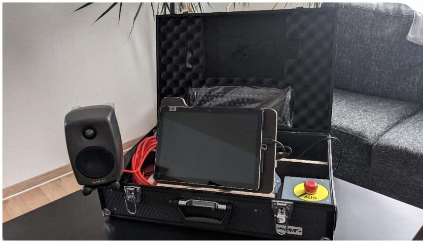
Figure 3. The test suitcase that all participants received from Hörzentrum Oldenburg, including all necessary equipment for remote fitting and testing of the Signia AX hearing devices.
