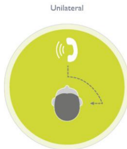
Figure 1. The phone signal is only routed to one ear in unilateral streaming.
